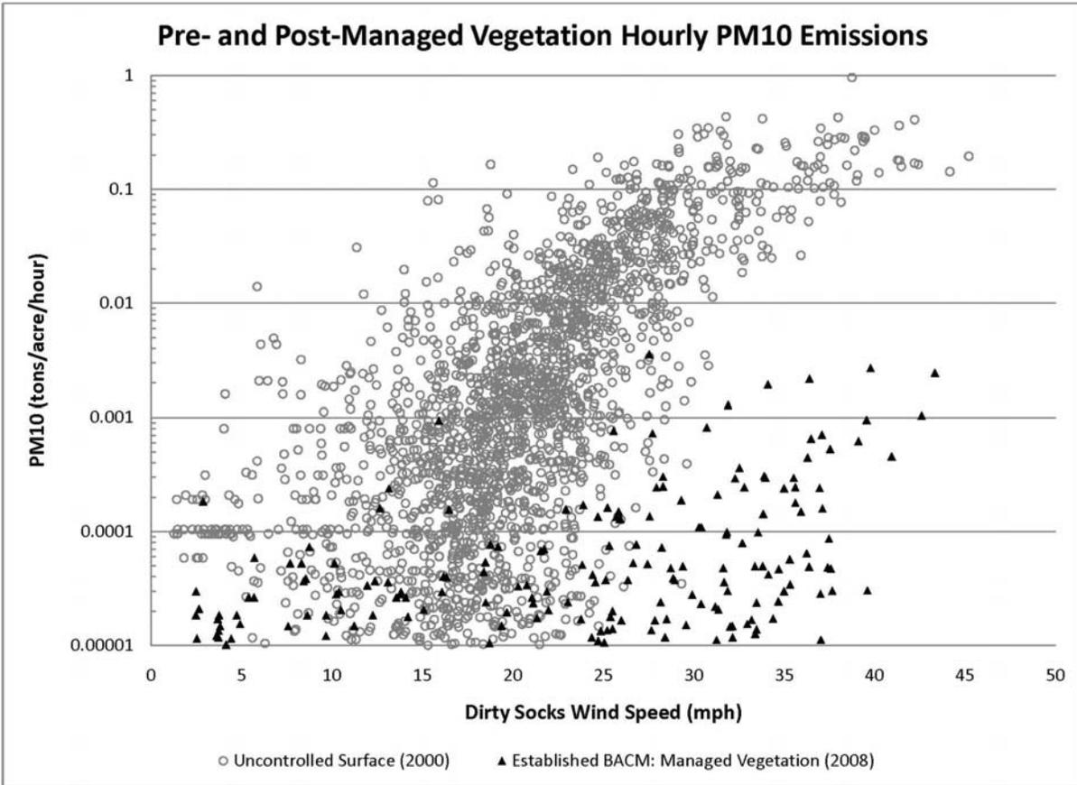
Figure 3. PM<sub>10</sub> emissions from the areas on Owens Lake on which the **Managed Vegetation** BACM was deployed. The graph shows emissions prior to and after BACM deployment. It can be seen that BACM generally reduced emissions at least 2 orders of magnitude or the 99% reduction required to meet the PM<sub>10</sub> standard.
