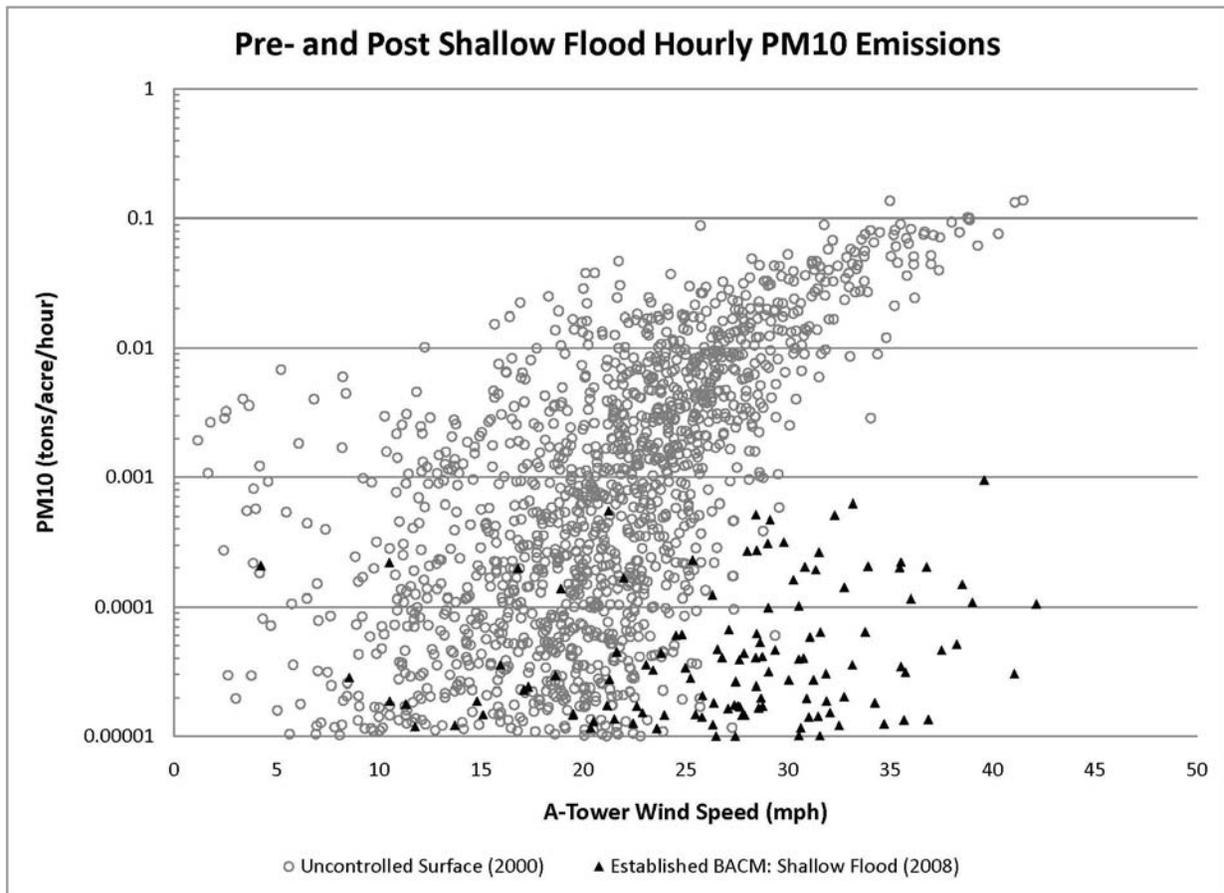
Figure 2. PM<sub>10</sub> emissions from the areas on Owens Lake on which the **Shallow Flooding** BACM was deployed. The graph shows emissions prior to and after BACM deployment. It can be seen that BACM generally reduced emissions by 2 orders of magnitude or the 99% reduction required to meet the PM<sub>10</sub> standard.
